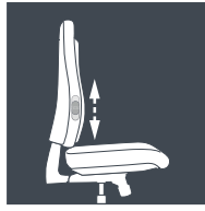
Backrest with integrated height adjustable lumbar support
